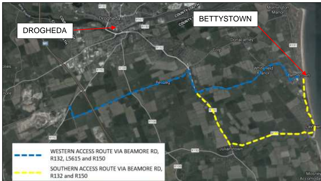
FIGURE 2.4: CONCRETE AGITATOR ROUTES TO BETTYSTOWN
