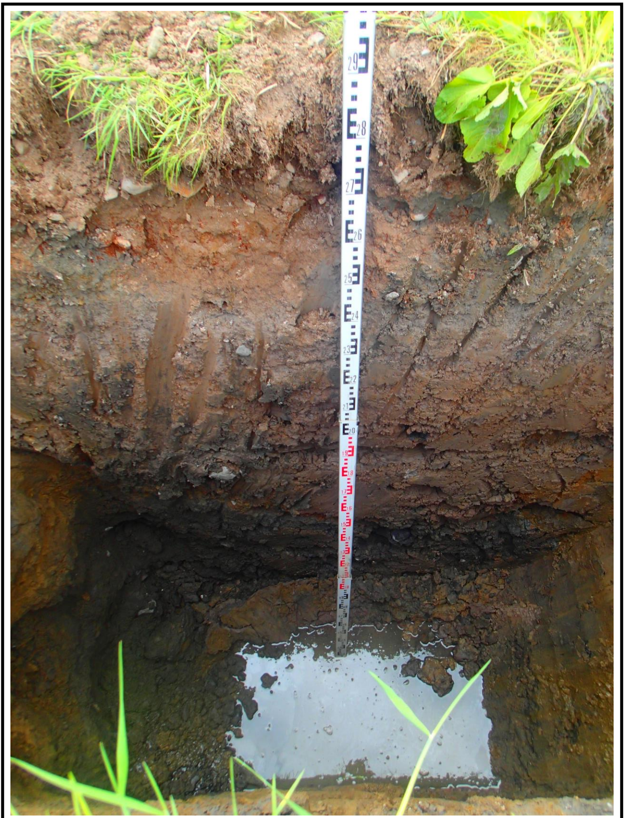
Plate A4: Profile of poorly drained topsoil overlying mottled very sandy gravelly SILT with occasional cobbles and boulders to 2.9m depth, in trial hole TP4. See the presence of the water table at the base of the hole.
