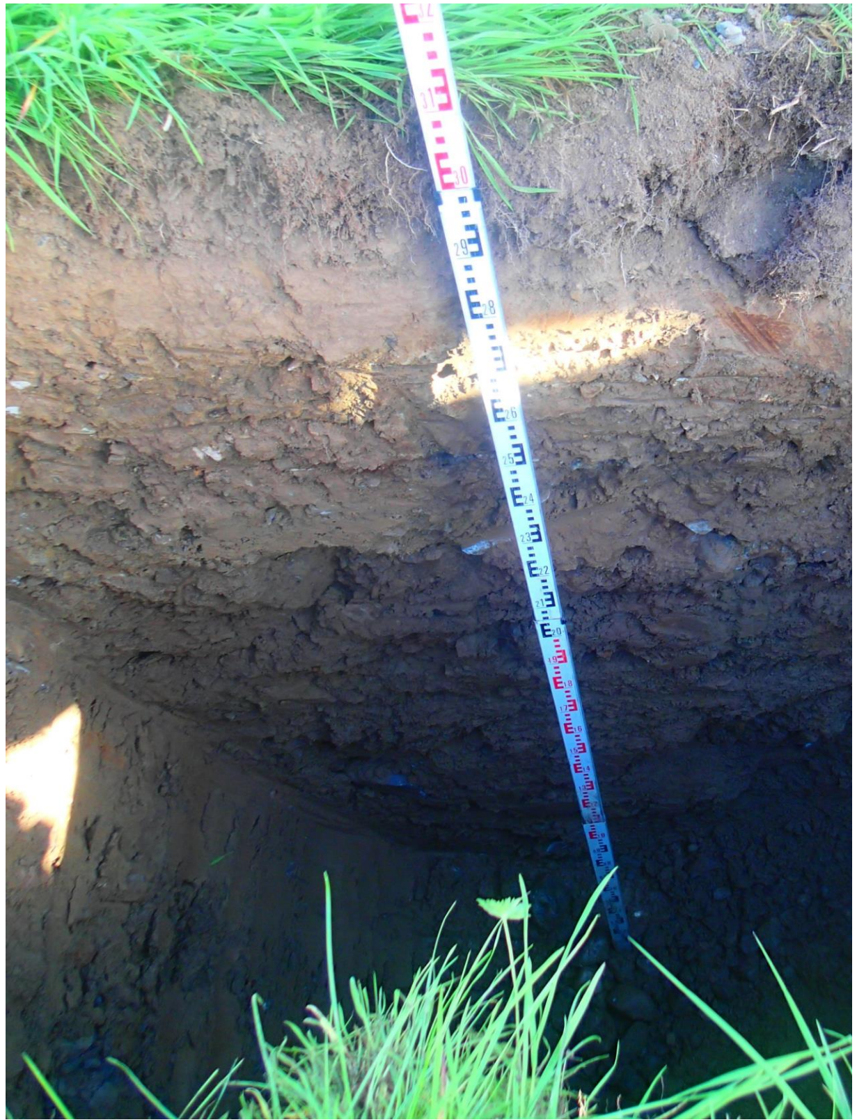
Plate A3: Profile of well drained topsoil overlying unmottled very sandy gravelly SILT with occasional cobbles and boulders to 3.05m depth, in trial hole TP3. See the absence of the water table and bedrock at the base of the hole.
