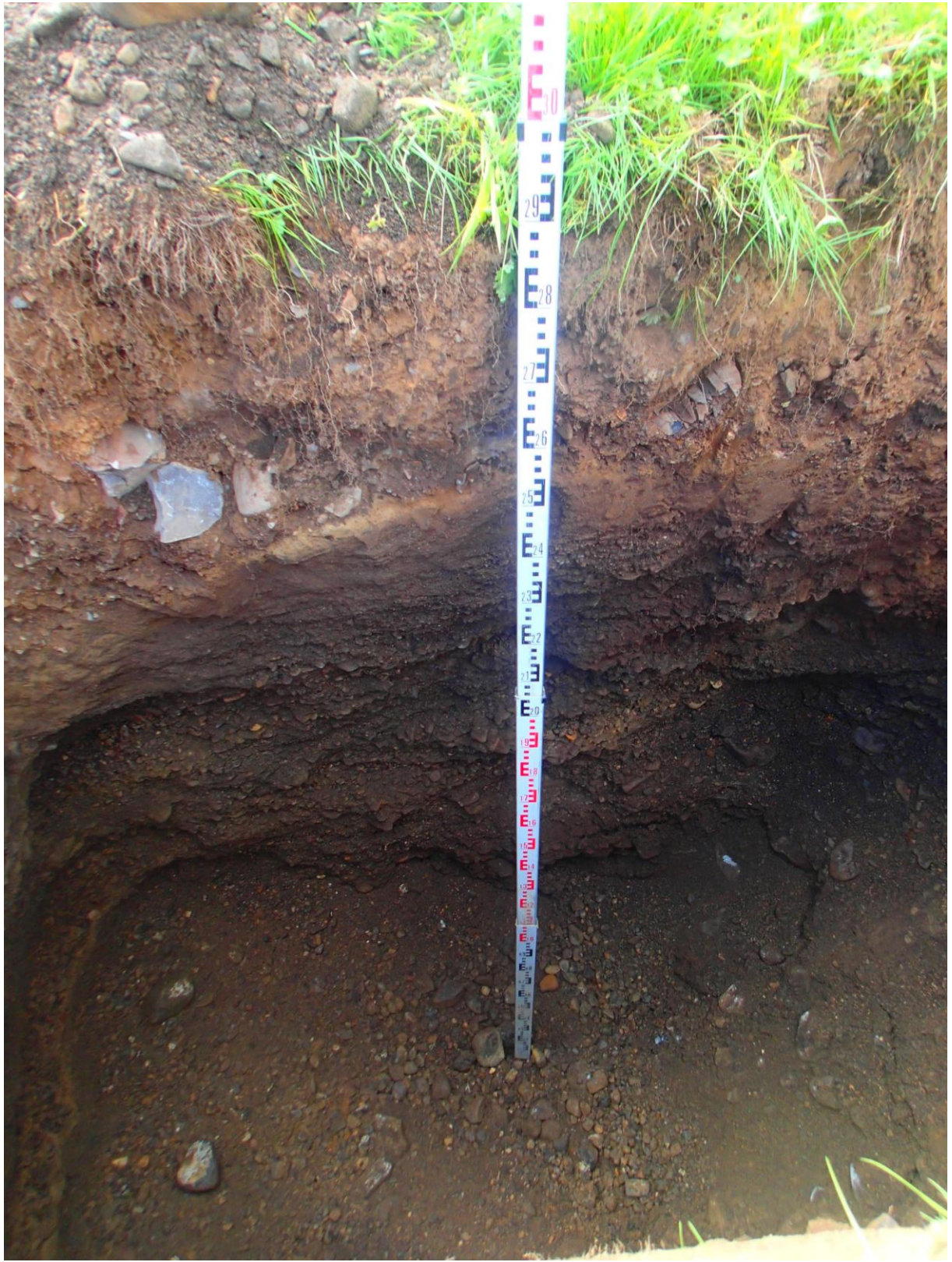
Plate A9: Profile of well drained topsoil overlying unmoistened very sandy gravelly SILT with occasional cobbles and boulders to 3.0m depth, in trial hole TP9. See the absence of the water table and bedrock at the base of the hole.
