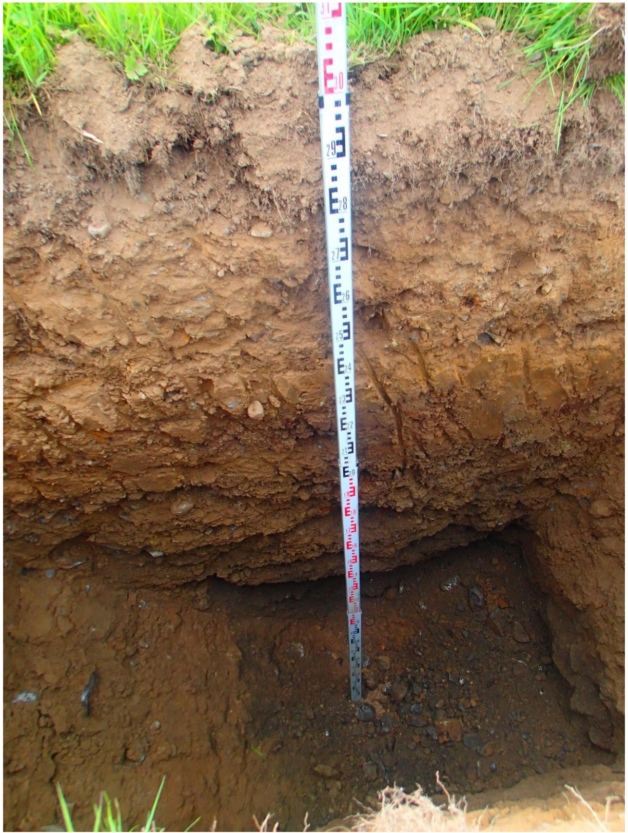
Plate A12: Profile of well drained topsoil overlying unmottled SAND with occasional gravels to 3.0m depth, in trial hole TP12. See the absence of the water table and bedrock at the base of the hole.
