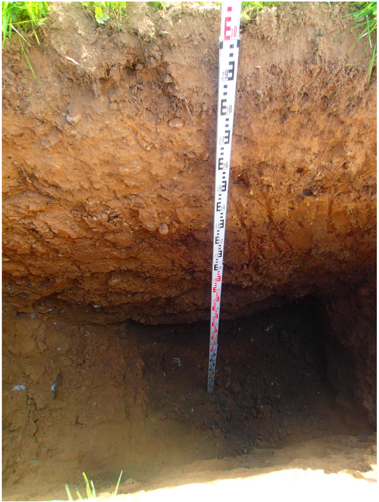
Plate A10: Profile of well drained topsoil overlying unmottled very sandy gravelly SILT with occasional cobbles and boulders to 3.0m depth, in trial hole TP10. See the absence of the water table and bedrock at the base of the hole.
