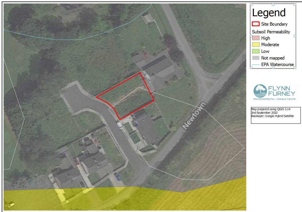
Figure 4 Subsoil permeability in the proposed works area
