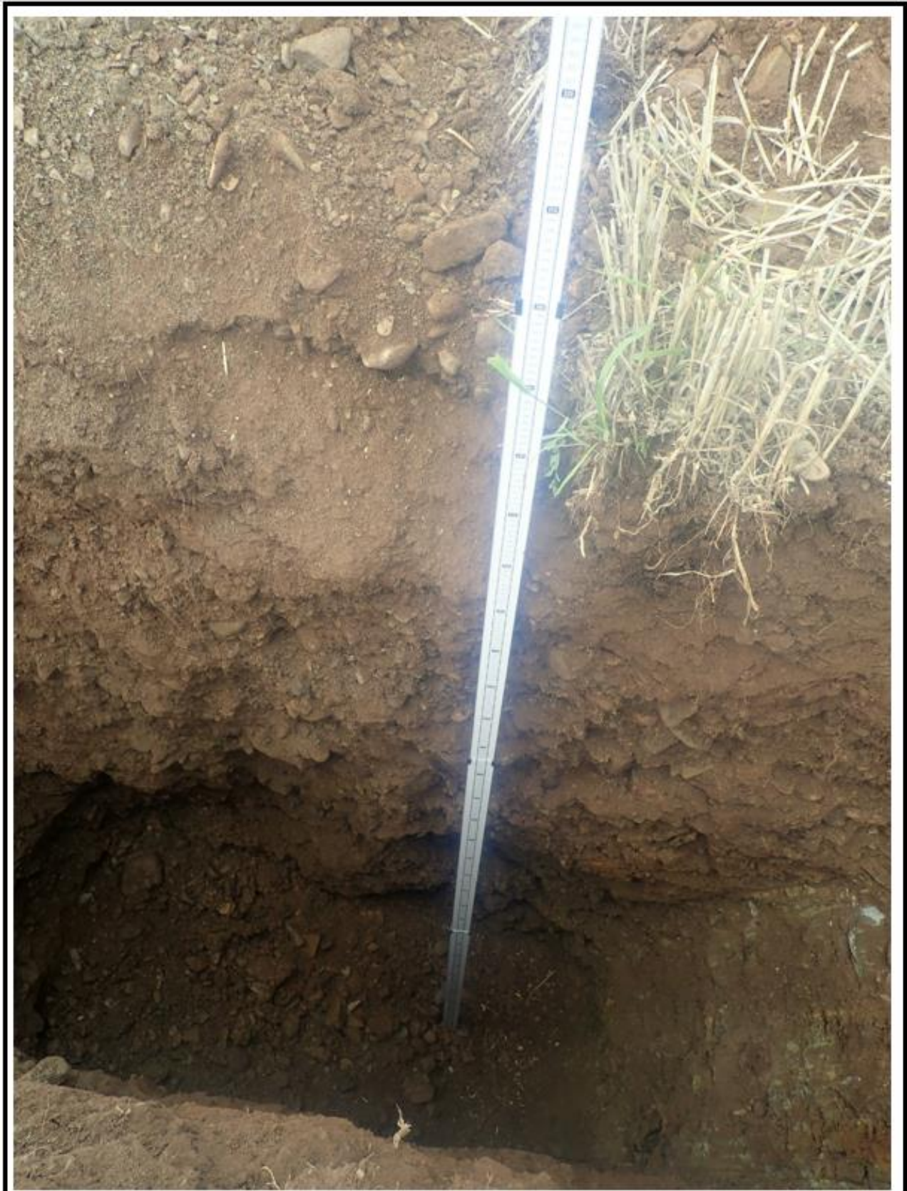
Plate A1: Profile of well drained topsoil overlying unmottled very silty sandy GRAVEL with occasional cobbles to 2.95m depth, in trial hole TP1. See the absence of the water table and bedrock at the base of the hole.
