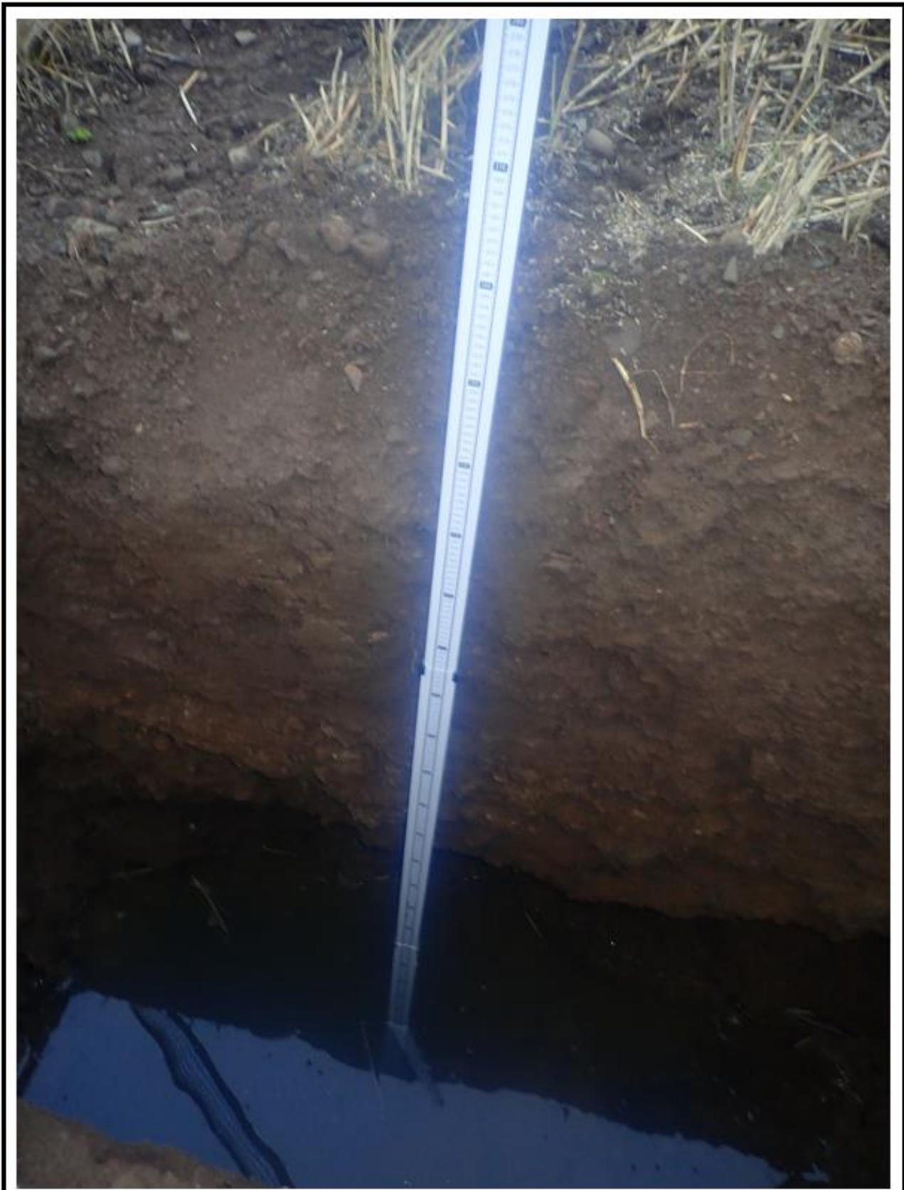
Plate A8: Profile of well drained topsoil overlying unstratified very silty sandy GRAVEL with occasional cobbles to 2.65m depth, in trial hole TP8. See the presence of the water table at 2.4m depth at the base of the hole.
