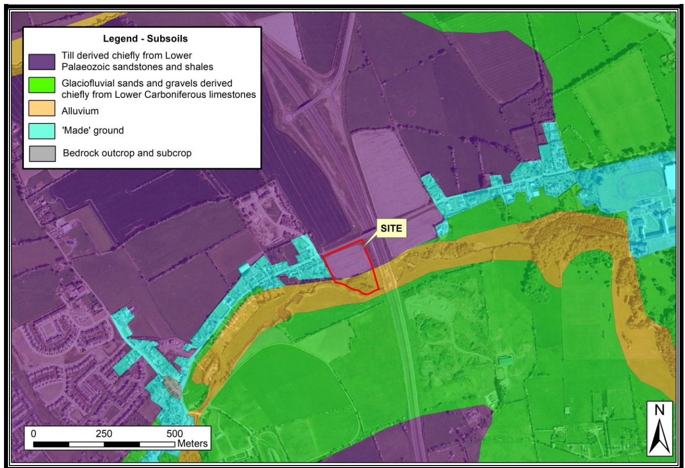
Figure 2: Subsoils geology of the site and its environs. The purple depicts till derived chiefly from Lower Palaeozoic sandstones and shales, the green depicts 'glaciofluvial sands and gravels', the orange alluvium, and the cyan 'Made' ground (OS Licence EN 0057922).
