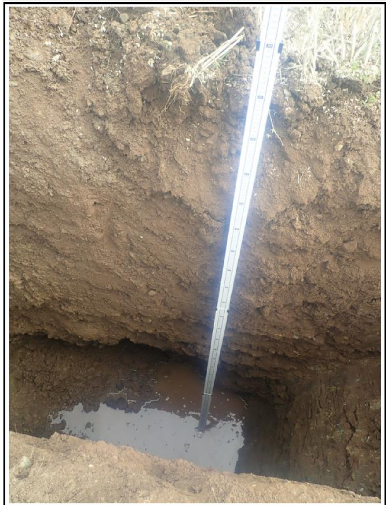
Plate A5: Profile of well drained topsoil overlying unmottled very silty sandy GRAVEL with occasional cobbles to 3.15m depth, in trial hole TP5. See the presence of the water table at 2.95m depth at the base of the hole.
