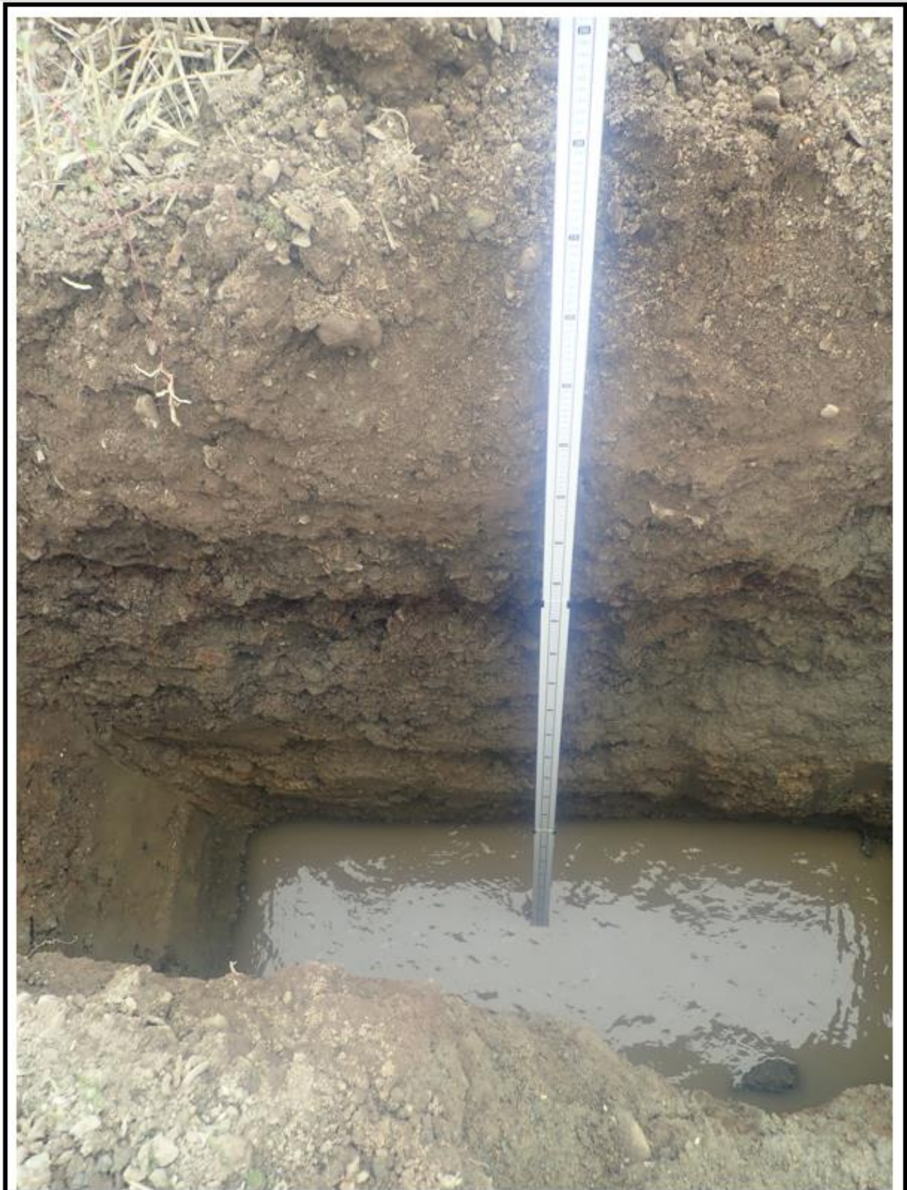
Plate A6: Profile of well drained topsoil overlying unmottled very silty sandy GRAVEL with occasional cobbles to 2.85m depth, in trial hole TP6. See the presence of the water table at 2.6m depth at the base of the hole.
