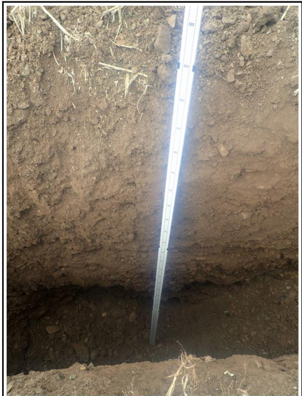
Plate A3: Profile of well drained topsoil overlying unmottled very silty sandy GRAVEL with occasional cobbles to 2.95m depth, in trial hole TP3. See the absence of the water table and bedrock at the base of the hole.
