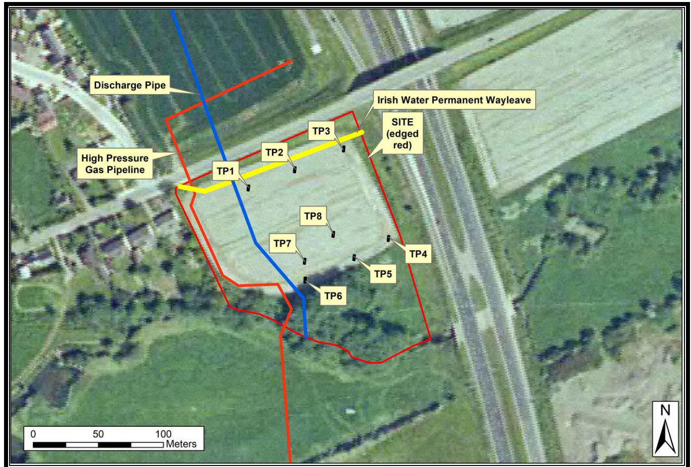
Figure 7: Location of trial pits excavated within the proposed Gormanston Townland, Stamullen burial ground site area, as well as infrastructure which had to be avoided during the dig process.
