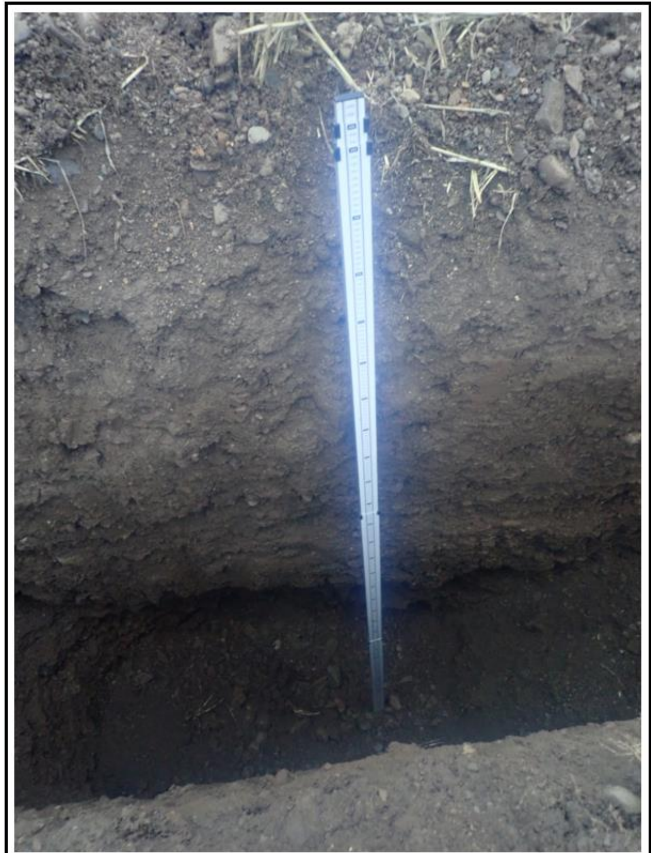
Plate A7: Profile of well drained topsoil overlying unmottled very silty sandy GRAVEL with occasional cobbles to 2.85m depth, in trial hole TP7. See the absence of the water table and bedrock at the base of the hole.
