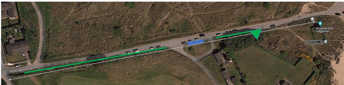
Map 6 Proposed New parallel parking and turning area (35 parking spaces, 3 disabled bays and a hammer head turning area)
