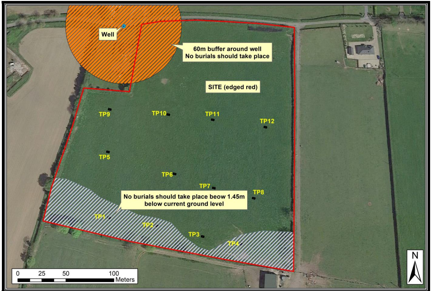
Figure 8: Plot showing wells around the site and the required 60 m buffer zones around these, given that the subsoil contains units of highly permeable sand and gravel. The only locality where burials can not take place on the site is within the stippled area at the northwestern corner.
