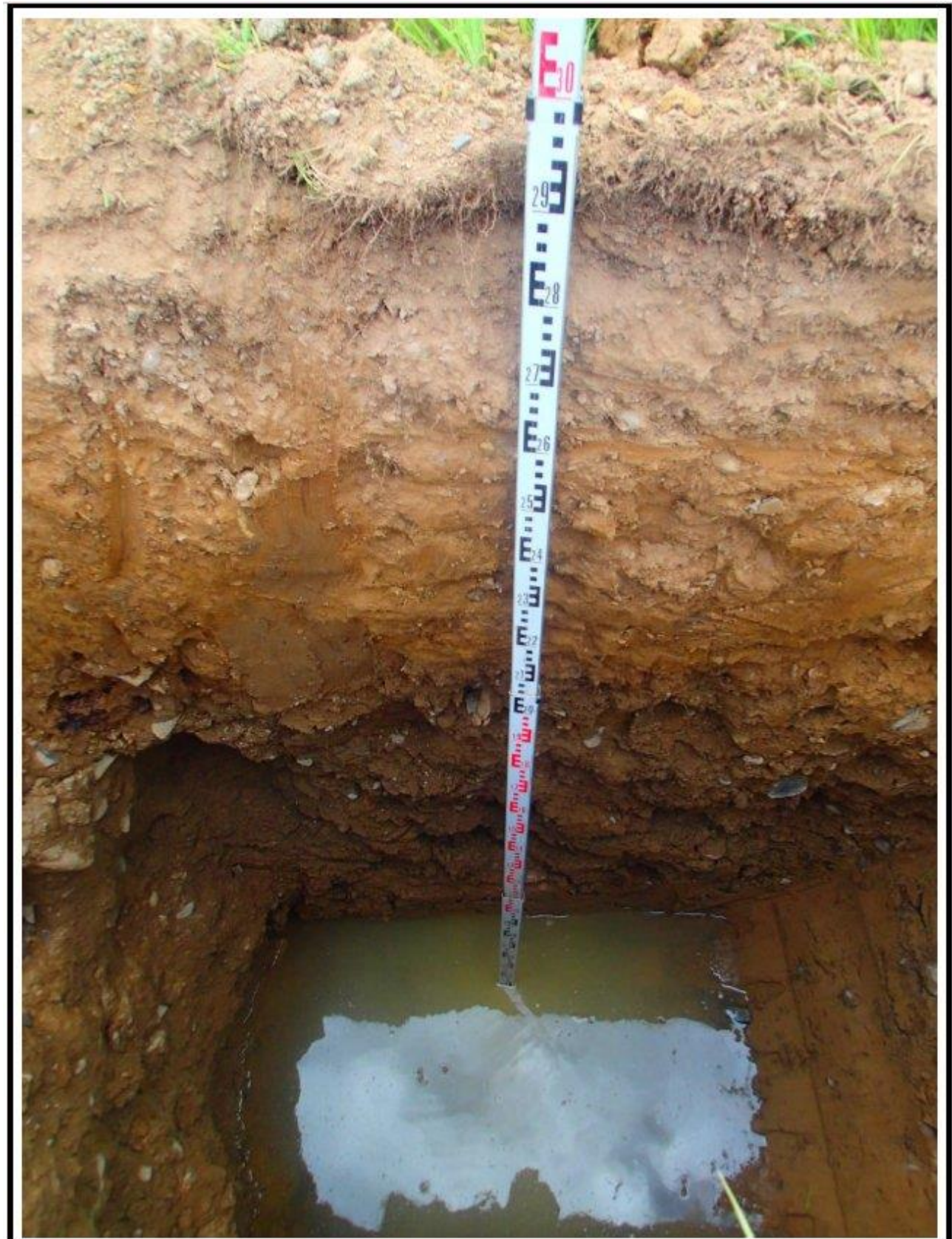
Plate A2: Profile of well drained topsoil overlying unmottled very silty gravelly SAND with occasional cobbles and boulders to 3.0m depth, in trial hole TP2. See the presence of the water table at the base of the hole.
