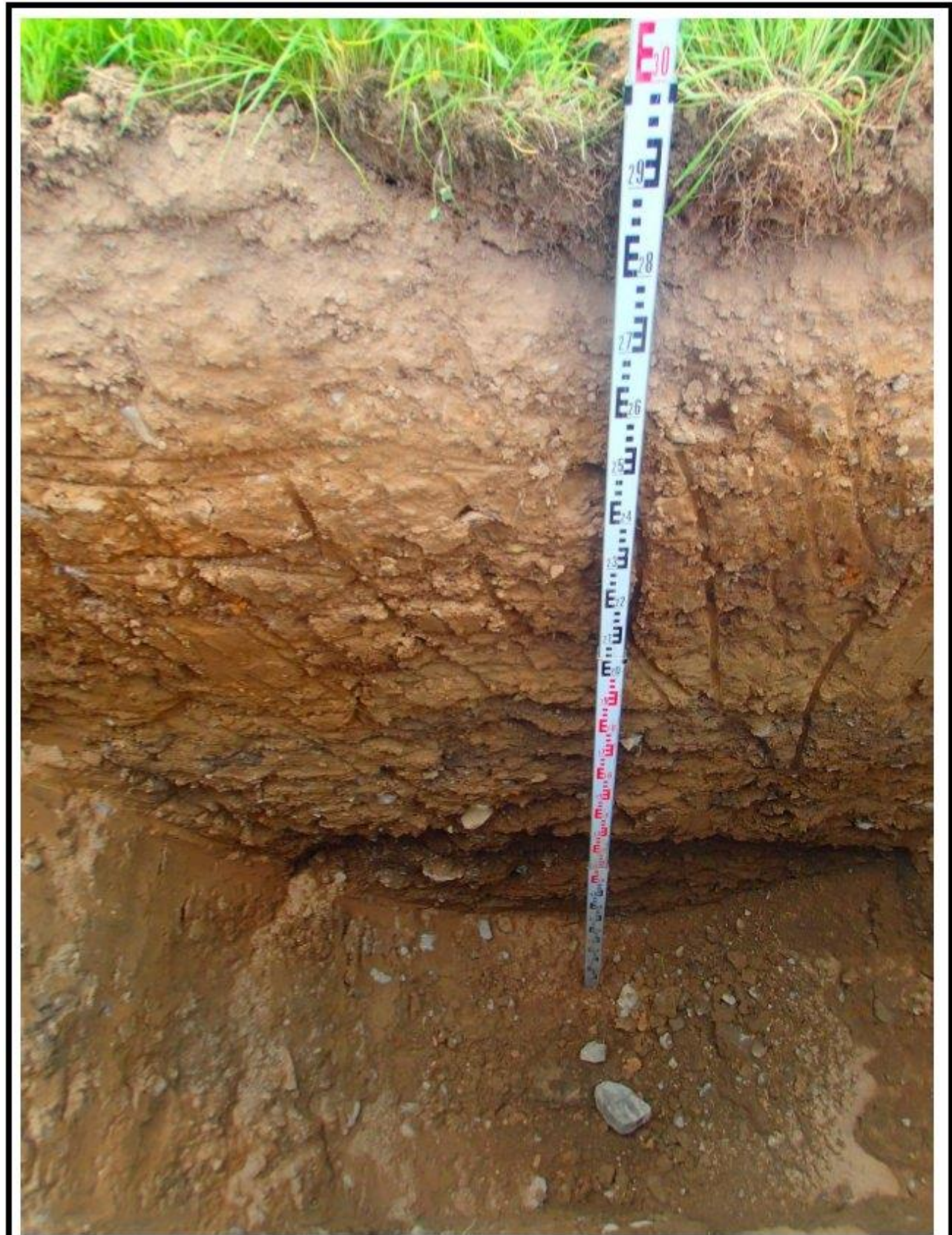
Plate A6: Profile of well drained topsoil overlying unmottled sandy SILT with abundant gravels and occasional cobbles and boulders to 3.15m depth, in trial hole TP6. See the absence of the water table and bedrock at the base of the hole.
