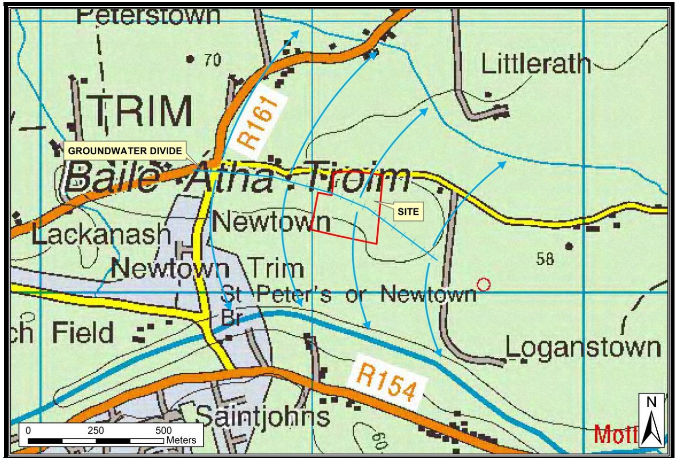
Figure 4: Interpreted groundwater flow directions under the land at Loganstown, using contours from the O.S. 1:50,000 Discovery Series map, levels measured on-site, and surface water stream flow directions. Flow should generally be towards the lower land to the northeast (in the northern section of the site) and towards the south (in the southern section, OS Licence EN 0057921).
