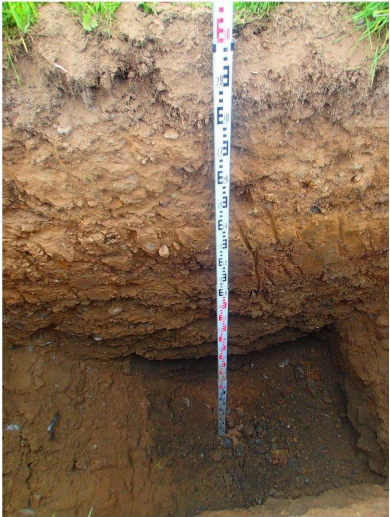
Plate A11: Profile of well drained topsoil overlying unmottled SAND with occasional gravels to 3.0m depth, in trial hole TP11. See the absence of the water table and bedrock at the base of the hole.
