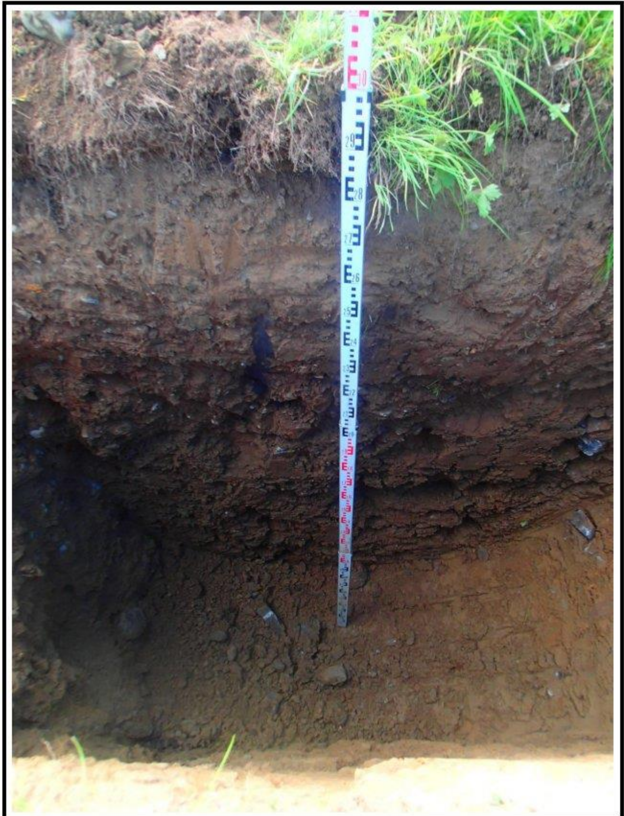
Plate A7: Profile of well drained topsoil overlying unmottled sandy gravelly SILT with occasional cobbles and boulders to 3.0m depth, in trial hole TP7. See the absence of the water table and bedrock at the base of the hole.
