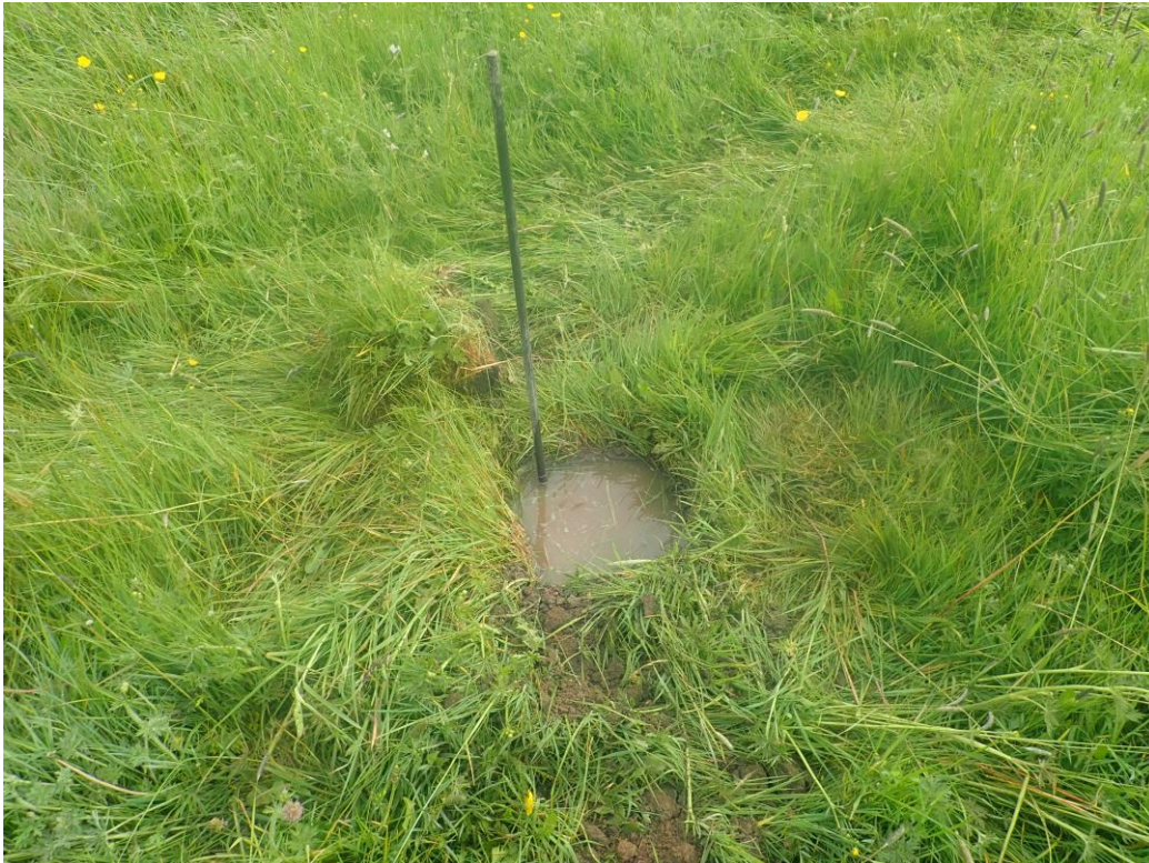
Plate 8: Water falling on morning of Wednesday 26 th May 2021 in surface test hole number 3.
