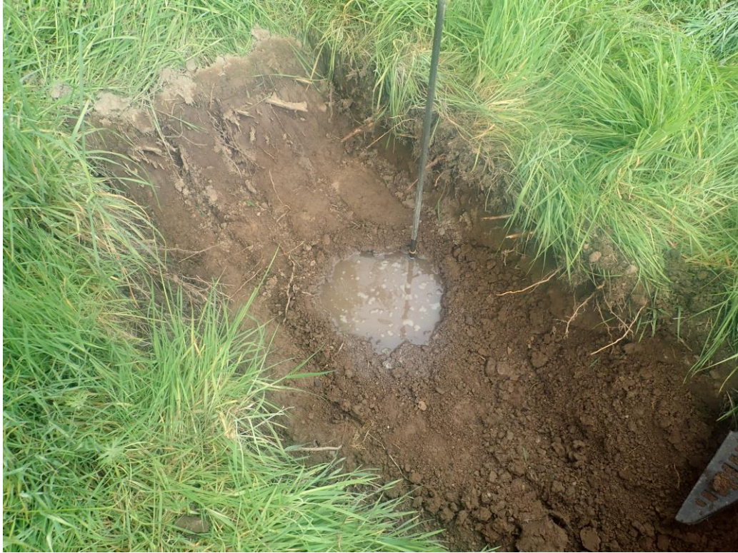
Plate 3: Water falling on morning of Wednesday 26 th May 2021 in subsurface test hole number 1.
