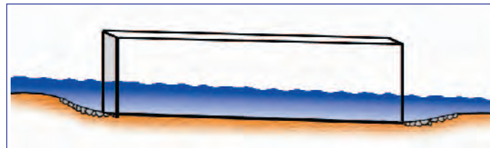
Fig. 2. Over-sized box culvert permanently backwatered
